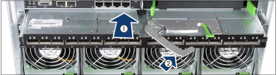
Figure 40: Installing a double-width connection blade
